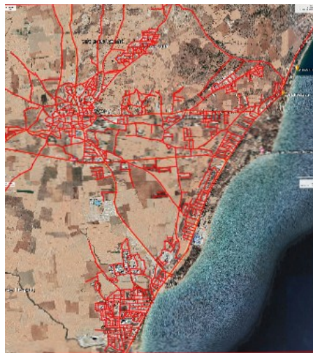
Figure 2: Axial Lines Generated in AutoCAD.
